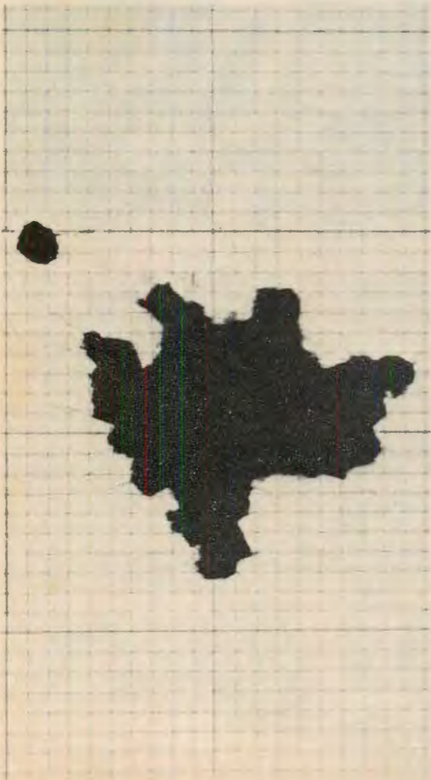
ABOVE: Standard military M1 ball through test barrel at 50 yards. Heavy squares are one inch, light squares are .1 inch. RIGHT: Tech. Sgt. Ernest F. Decker, 33, reloads Beretta 92S-1. Note dropping of spent magazine. BELOW: Ragged hole was cut by 100 rounds of flat-nose ball through test barrel at 50 yards.
